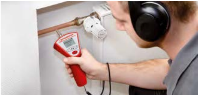
Acoustic leak detection of heating installations
