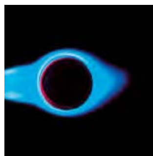
High flame temperature based on cyclone swirl
