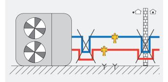
Freezing protection valves must be installed:
