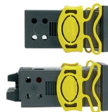
The 230 Vac model fitted with built-in transformer is the most compact model in the range (just 56.5 mm deep). This is undoubtedly a significant advantage in applications where the space available to house the controller is limited.
