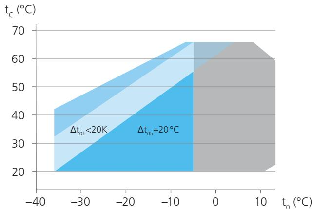
$t_0$  Evaporating temperature (°C)
