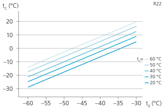
R22     $t_u$  Subcooling temperature at the intermediate cooler outlet
