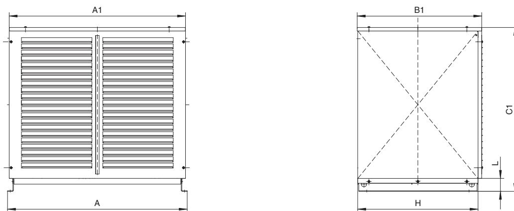
A1, B1, C1: Dimensions of the appropriate weather protective housing
